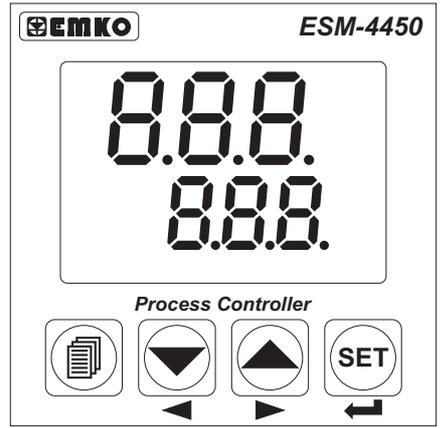
Third segments of top and bottom displays are tested.
