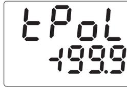
Minimum value for selectable dual point calibration
