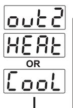
**Con2** It defines control algorithm of output module in Module-2 socket. It is active if output function of Module-1 is heating or cooling.
