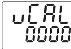
**Voltage / Current Input Calibration Type Selection**
