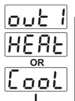
**Con 1** Defines control algorithm of output module in Module-1 socket. It is active if output function of Module-1 is heating or cooling.
