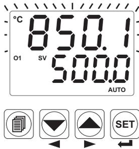
5 - If top display blinks : If analogue input value is greater than maximum value of operating scale  $\boxed{uPL}$  , top display starts to blink.
